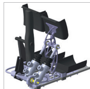
Fig. 4 Topology optimized brake pedal inside the pedalbox © TU Graz Racing Team
