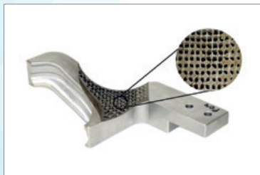
Fig. 5: Tong with a structure that is adapted to the production process and loads
