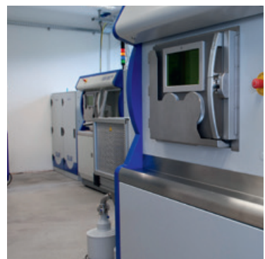
Fig. 3 View into the production hall: Additive manufacturing using two SLM®280 machines and one SLM®500 machine
