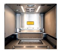
The **high-performance machine** is available in several configurations, providing single optics (1x 400 W or 1x 700 W), dual optics (1x 700 W and 1x 1000 W) and twin optics (2x 400 W or 2x 700 W). Depending on how the parts are arranged, a 80 % higher build rate can be achieved. In addition, the **patented bidirectional powder coating** helps to reduce the manufacturing time of individually manufactured metal parts.
