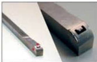
▶ Welding of openings with little distance of the edges
