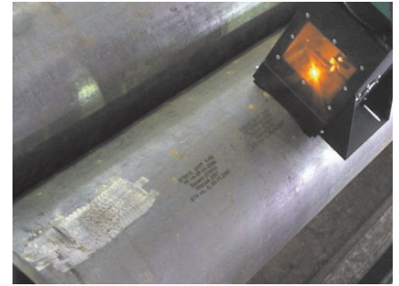
Marking of steel pipes
