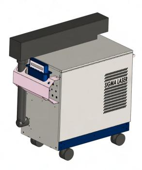
Laser beam source Nd.YAG: available with 120, 160 and 300 Watt output power and up to 20 meter fiber optic cable.
